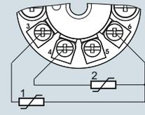
Mean-value/differential or redundancy generation 2 x two-wire system <sup>1)</sup>
