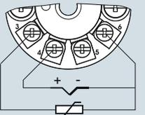
Cold junction compensation with external Pt100 in two-wire system <sup>1)</sup>
