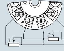
Mean value, differential or redundancy generation 1 resistor in two-wire system <sup>1)</sup>
