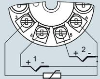
Mean value, differential or redundancy generation and cold junction compensation with internal Pt100 in two-wire system <sup>1)</sup>
