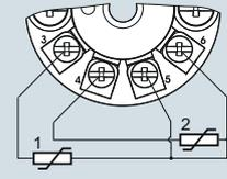
Mean-value/differential or redundancy generation 1 sensor in two-wire system <sup>1)</sup>
